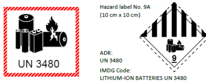
Figure 3. Left, label for stand-alone batteries with a nominal energy \leq 100 Wh. Right, label for stand-alone batteries with nominal energy > 100 Wh
